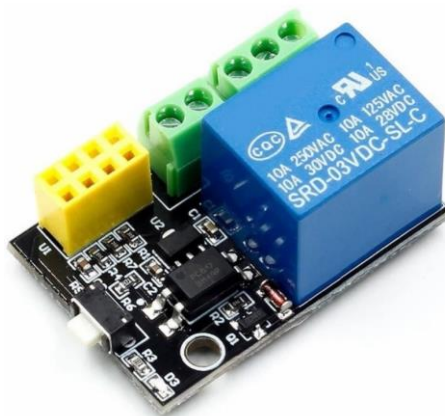
Figura 9 – Shield relé ESP8266 ESP-01 [16].
